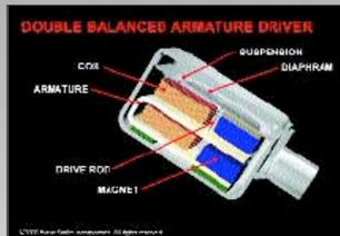
Figure 2: The inner transducer workings of the armature transducer design
