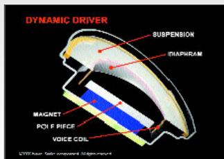
Figure 3: The dynamic driver really looks like a regular loudspeaker, only smaller.
