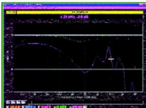
Figure 1: The dual armature is green and the single dynamic is purple. Note the dramatic rolloff on the high-end frequencies.
