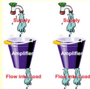
Image 1: Don't kick the bucket! Two loudspeakers in parallel require twice the current of a single one, just like two holes in a bucket offer one-half the opposition to water leaving the bucket as a single one.
