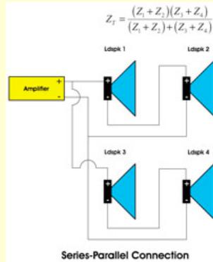
Series-parallel is useful within loudspeaker enclosures to allow a target impedance to be achieved with multiple devices.
