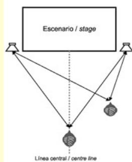
Figure 1: When the distance to both sides is the same, sound from both sides arrives at the same time. As we are closer to one side and farther from the other, sound from one of the sides arrives before the other.
