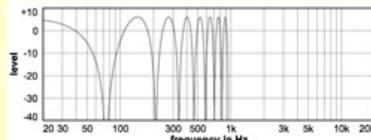
Figure 2: Frequency response of two signals spaced 7 milliseconds in time.
