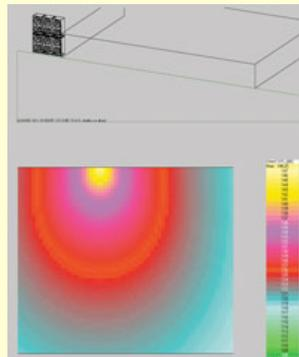
Figure 3: Single subwoofer side, modeled at 100 Hz.
