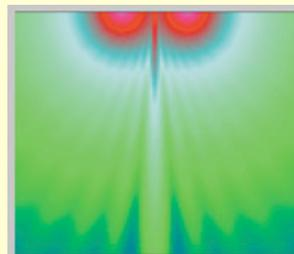
Figure 7: The power alley that results with two sub stacks spaced 47 feet apart.
